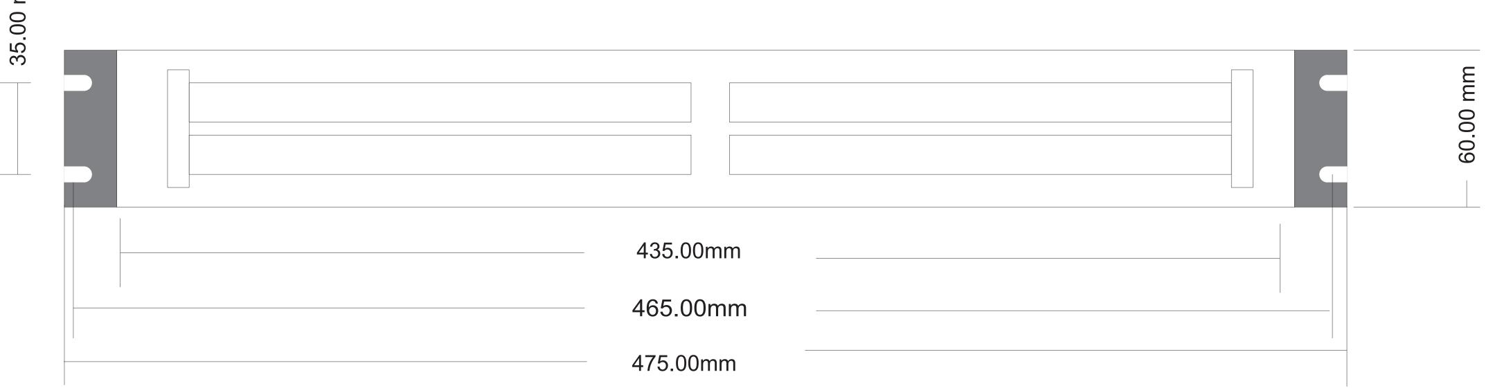
Tolerance:Limit Dimensions for linear measurement (mm) to DIN ISO 2768 -1m
